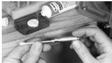
RIFLE DIES ONLY Be sure to lube the inside of the case neck with a cotton swab.
