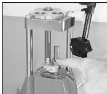
RIFLE DIES ONLY Be sure to lube the inside of the case neck with a cotton swab.
