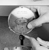
With the cover on use a pencil to hold the primers in the tray while assembling it to the priming tool. Shake the unit side to side
