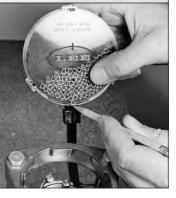
Place no more than 100 CCl or Winchester brand primers in the tray. (Use of any other brand exposes the operator to unnecessary risks.) With the cover off, shake side to side to turn all primers right side up.
