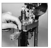
3 Lower the lever, and the powder measure will automatically charge the case while expanding the case mouth to accept the bullet
