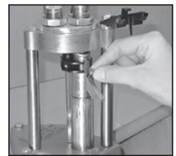
3 SELECT THE CORRECT LEVER PRIME ASSEMBLY (large or small). With clean fingers, place the correct size and type of primer in the primer guide. (This operation is greatly speeded by using the Lee Safety Prime primer feeder. Never touch the primer from box to shell.) Seat the primer by lowering the ram—lifting up on the press lever. Lift firmly enough to seat the primer flush to slightly below flush of the case head.
