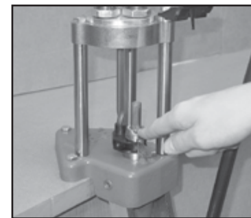
2 SIZE THE CASE Place a shell in the shell holder. Rotate the turret to position the full length sizer over the case. Firmly raise the ram to the top and stop.
