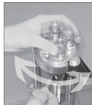
4 FLARE CASE MOUTH for ease of bullet installation. Raise the ram to expand the case neck. To increase the flare, screw the die in deeper. Always adjust to provide the minimum flare needed to start the bullet. After proper adjustment, tighten the lock ring.
