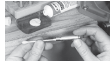
RIFLE DIES ONLY Be sure to lube the inside of the case neck with a cotton swab.
