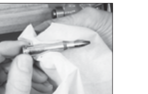
6 IF LOADING maximum loads, it's good practice to remove all traces of case lubricant with detergent and water. This will reduce pressure against the bolt.
